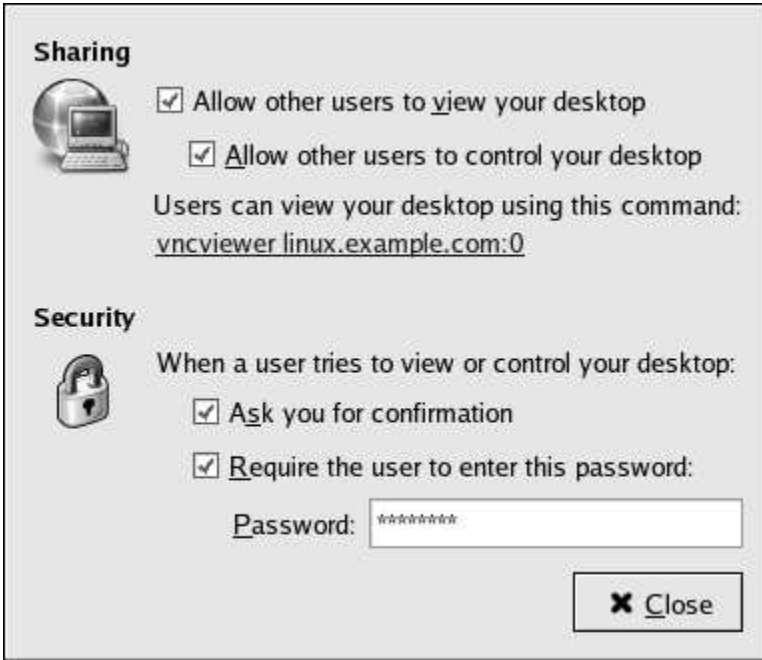
Figure 5-2. Remote Desktop Access for Administration
